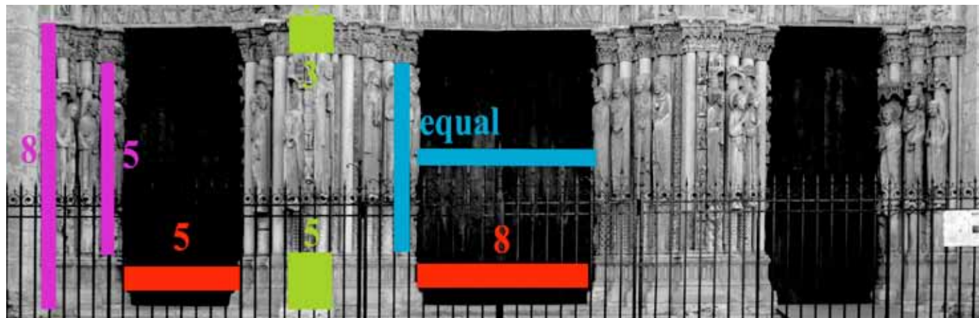
Weaving proportions across the major elements of the portal, first scheme Master-11.
